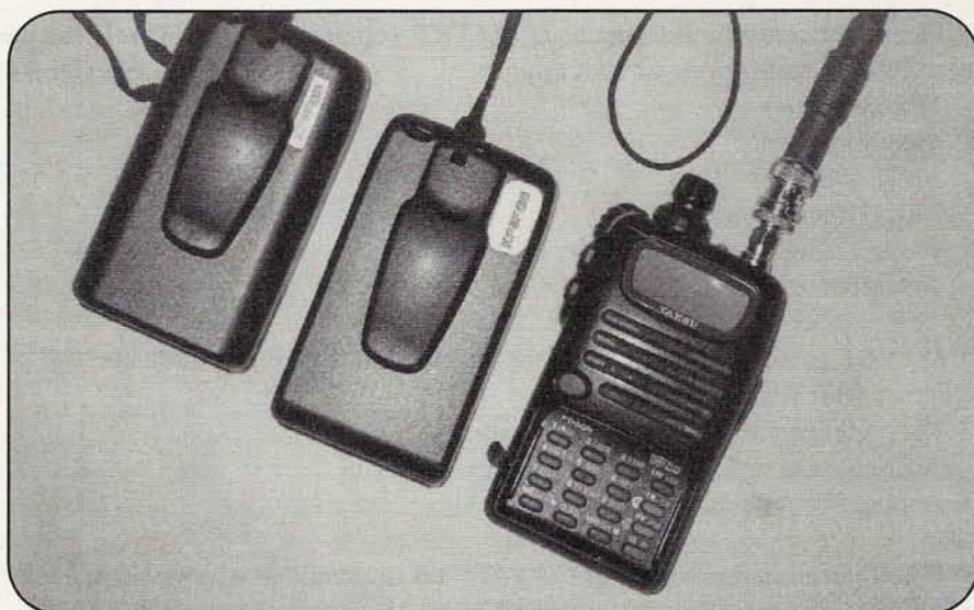
Photo A. The author's HT shown with stock NiCd batteries. Getting an extra battery pack will extend your "talk time," but won't give you higher output power. (Photos by the author)
