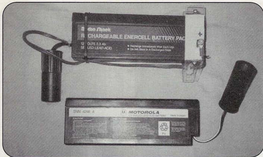
Photo B. Two different 2.3-AH (amp-hour) batteries. Top: replacement camcorder battery with homemade clamp; bottom: commercially available gel-cell with built-in accessory jack.
