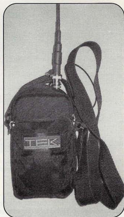
Photo F. A camera case also serves well to carry an HT in the back pocket and a battery pack in the front.
