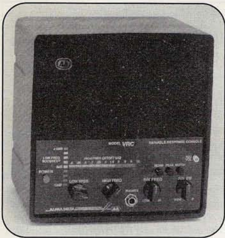
Photo A. If you appreciate great audio and want your rig to sound as good as a big home stereo, cable one of these Alpha Delta VRC speaker systems to its output. The unit features adjustable bass/treble equalization, a ducted port bass reflect speaker, and can make your home or mobile station sound like a recording studio. Photo courtesy Alpha Delta Communications, Inc.
