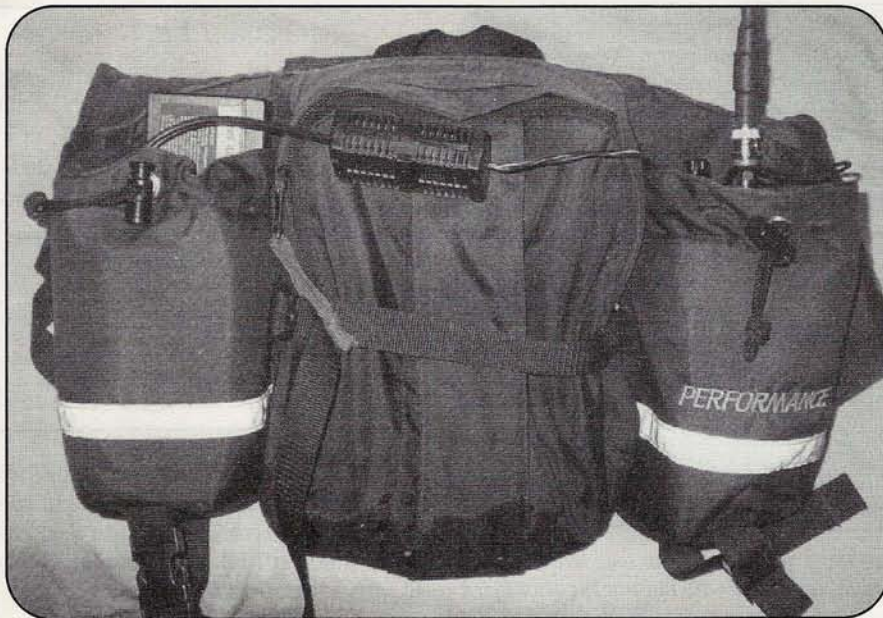
Photo E. Bicyclist's fanny pack designed to hold two water bottles can also hold radio gear. In photo, the HT is in the right pocket and a 2.3-AH cell is in the left pocket, connected together with 12-volt adaptor. The center pocket is available for carrying anything else, such as spare battery, lunch, or maps.
