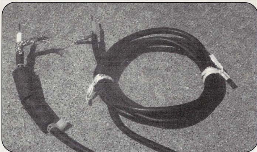
Photo B. Two different ways of making a 6-meter "noise balun" (see text) to keep RF from running back up the outside of the feedline. On the left, two big ferrite beads do the job, while the balun on the right uses three or four turns of the coax itself to create an RF choke.
